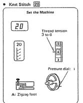
Set the Pressure Dial to "1", so that the knit will retain its shape as you are sewing.
